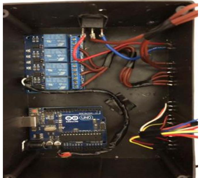
Fig 9. Installation relays and Arduino to the panel.
